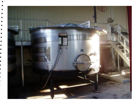
One of the custom fermenting tanks designed by Ed Gomez at Russian Hill Winery There are actually cooling units (not visible) on the bottom of the tank to aid in precise control of temperature during fermentation.
